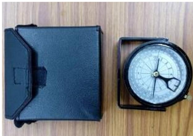
**Fig . 4.1 Clinometer – Compass**
